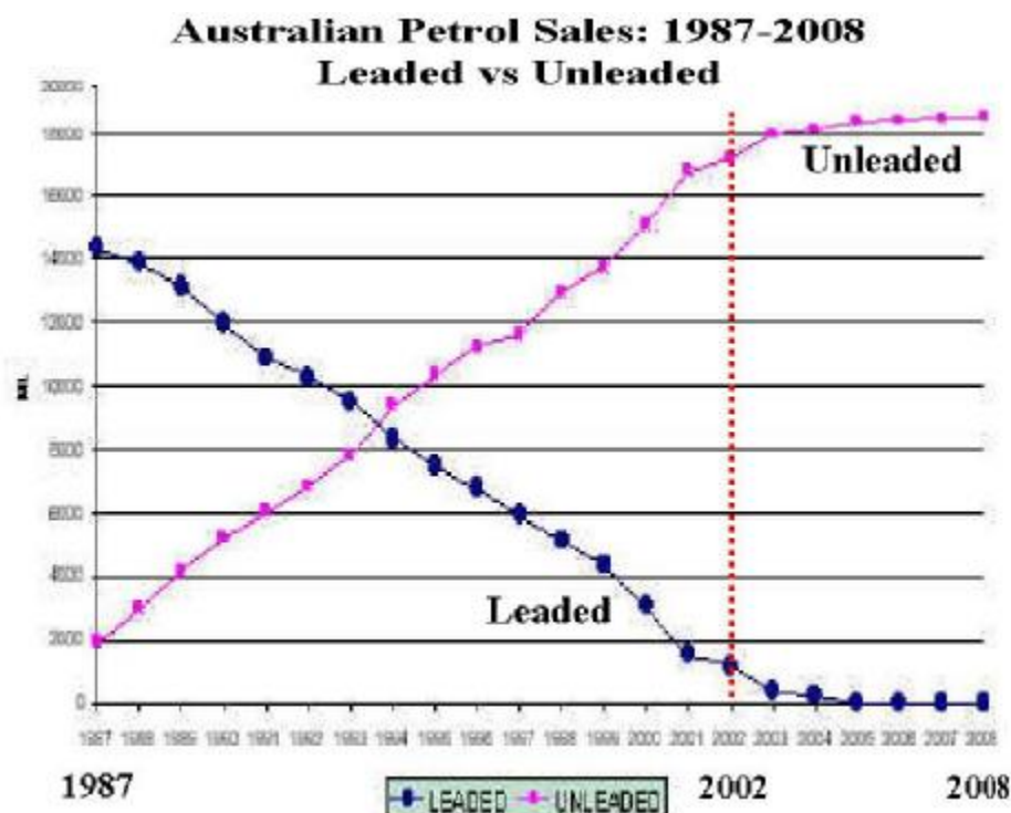
Fig. 7. Example of the inevitably slow rate of introduction of new technology into Australia's vehicle fleet. Unleaded and leaded (or LRP) petrol sales, Australia, from 1987 and extrapolated to 2008, (Australian Institute of Petroleum at www.aip.com.au ), following mandatory introduction of emission-control engines in new cars in 1986. The introduction of hybrid vehicles and fuel cells is likely be much slower as the technological differences are much greater.
